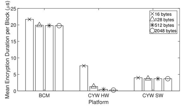
Fig. 7. This graph depicts buffer size (bytes) versus mean encryption duration per block ( $\mu s$ ) for 128-bit key size. As buffer size increases, CYW HW's encryption duration becomes much lower than the other platforms'. BCM SW sees a slight reduction in duration and all other variants remain relatively unchanged.
