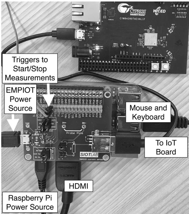
Fig. 1. Components of the EMPIOT Energy Measurement Platform
