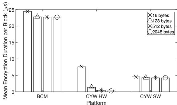
Fig. 8. This graph depicts buffer size (bytes) versus mean encryption duration per block ( $\mu$ s) for 192-bit key size. As buffer size increases, CYW HW's encryption duration becomes much lower than the other platforms'. BCM SW sees a slight reduction in duration and all other variants remain relatively unchanged.
