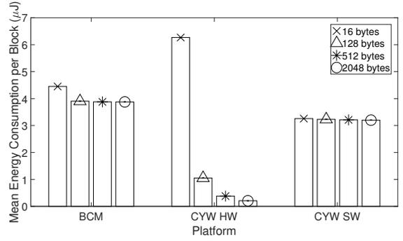
Fig. 4. This graph depicts buffer size (bytes) versus mean energy consumption per block ( $\mu\text{J}$ ) for 128-bit key size. As buffer size increases, CYW HW's energy consumption becomes much lower than the other platforms'. BCM SW sees a slight reduction in cost at the smallest buffer sizes while the rest of the implementations remain relatively unchanged.
