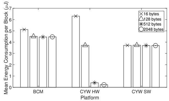
Fig. 5. This graph depicts buffer size (bytes) versus mean energy consumption per block ( $\mu\text{J}$ ) for 192-bit key size. As buffer size increases, CYW HW's energy consumption becomes much lower than the other platforms'. BCM SW sees a slight reduction in cost at the smallest buffer sizes while the rest of the implementations remain relatively unchanged.
