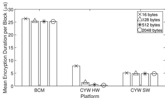
Fig. 9. This graph depicts buffer size (bytes) versus mean encryption duration per block ( $\mu$ s) for 256-bit key size. As buffer size increases, CYW HW's encryption duration becomes much lower than the other platforms'. BCM SW sees a slight reduction in duration and all other variants remain relatively unchanged.
