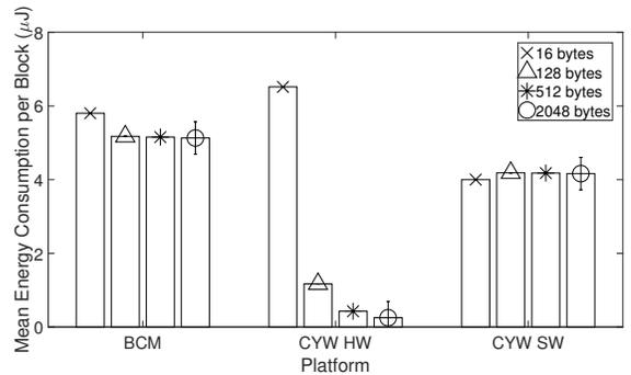
Fig. 6. This graph depicts buffer size (bytes) versus mean energy consumption per block ( $\mu\text{J}$ ) for 256-bit key size. As buffer size increases, CYW HW's energy consumption becomes much lower than the other platforms'. BCM SW sees a slight reduction in cost at the smallest buffer sizes while the rest of the implementations remain relatively unchanged.
