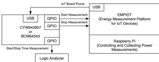
Fig. 2. Interconnection with the EMPIOT Energy Measurement Platform
